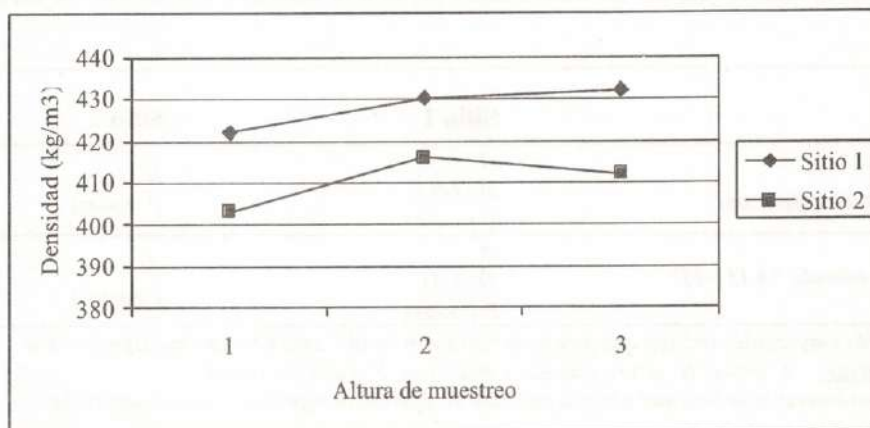
Graphic 1. Basic density ( \text{kg/m}^3 ) mean values by sampling height for american willow in sites 1 and 2.
