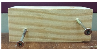
Figure 2. Test specimen in the radial direction with two screws placed more than 50 mm apart
