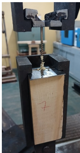
Figure 3. Test specimen under testing in the universal machine
