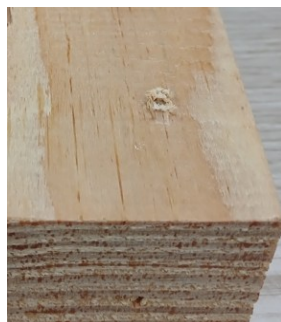
Figure 5. Insertion across the tangential direction intersects earlywood and latewood bands
